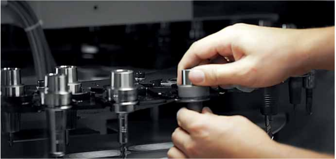
Double-row HSK-E40 magazine internal to the machine's standard footprint with a capacity of 68 tools.
