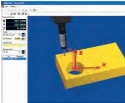
JMS® Pro PreSet 3D the presetting software with user guidance and automatic data recording in JMS® Pro.
