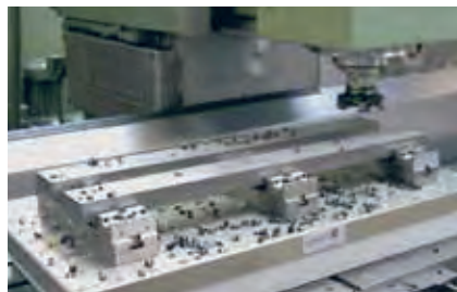
ClampSet also for long and big workpieces.
