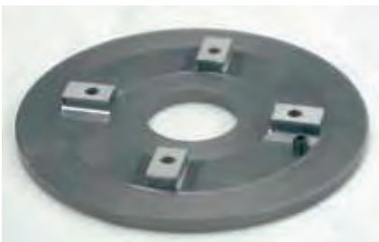
The flat precision pallet is the basis for all clamping processes.
