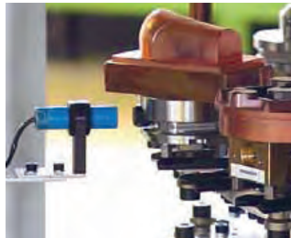
The EWIS™ Rapid identification system provides an overview of holders and pallets. With the modern transponder chips, every pallet can be identified at any time. The handling facilities examine the magazine loads automatically.
