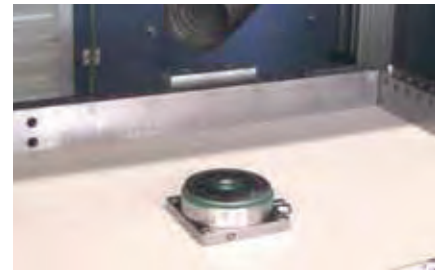
The chucks can be fitted to the machine table directly or with adapter plates.
