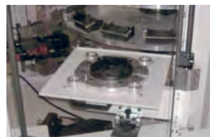
Loading station for user-friendly loading/unloading cycles.
