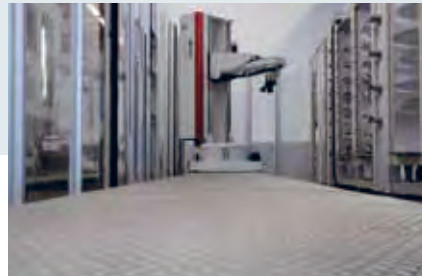
02 | The stable linear rail is extended to the required length in segments.
