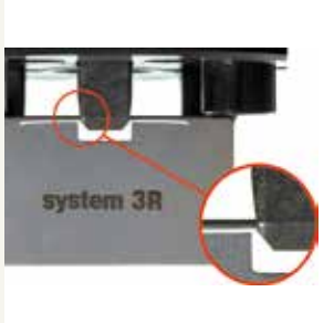
The lip edge of the pallet is angled to match the angle of the boss. This maximises the mating surface area between the parts, resulting in precision alignment, minimal wear and enduring precision.
